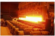
A door being opened to retrieve a reheated steel slab.
