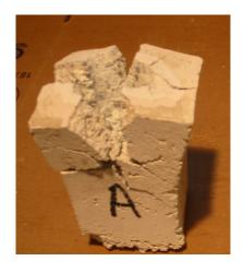
This sample shows what happens when alkali reacts with alumina to form beta alumina. A very expansive reaction that is destructive to the refractory.
