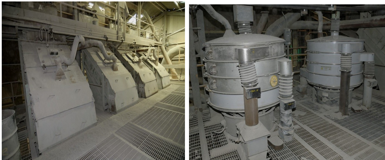
Pictured above are the two-step screening stations at the Curwensville plant, allowing the plant to size raw materials and keep costs to a minimum.
