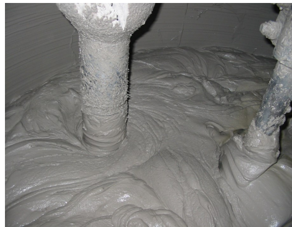
High intensity mixing as supplied by an Eirich mixer is essential to having a smooth easy to use mortar.
