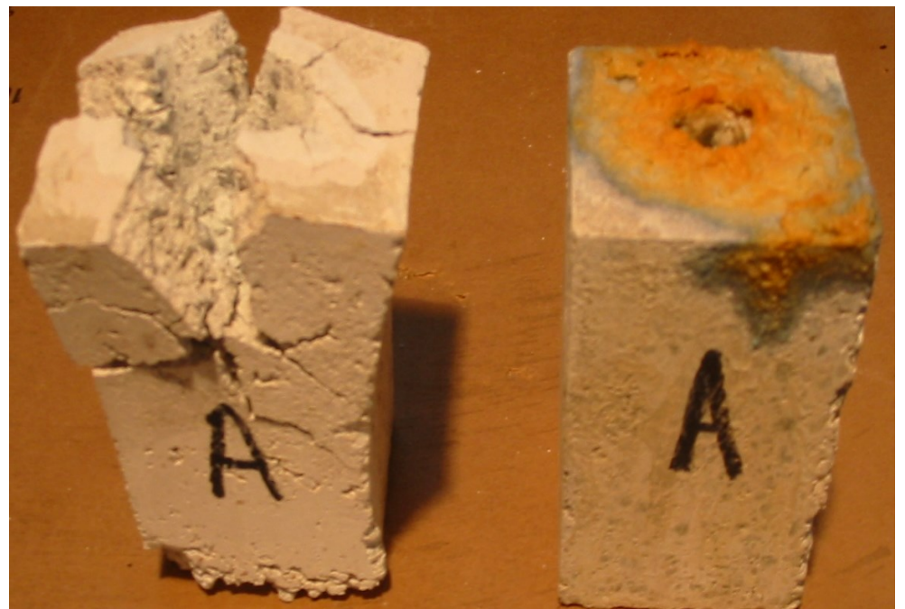
Alkali test samples after 4 cycles at 1800°F. The standard sample on the left broke apart while the SAVAGE X 60 GM material on the right is unaffected.
