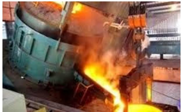
**An electric arc furnace (EAF) teeming into a steel ladle. Production of both EAF steel and integrated steel is down country wide.**
