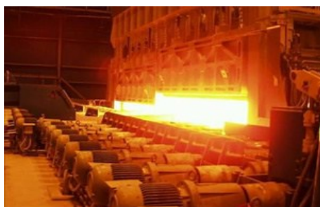
A door being opened to retrieve a reheated steel slab.
