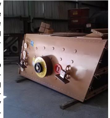
This three stage screen deck is now screening operating 4 stories above the plant floor
