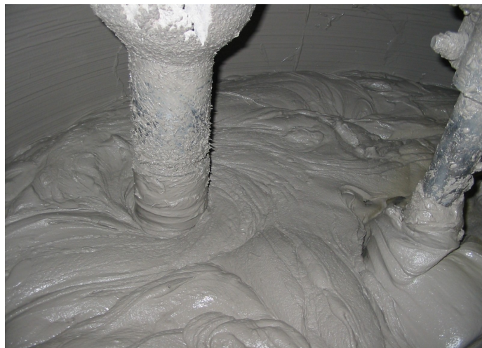
The best mortars are made in high intensity mixers such as this Eirich Mixer at Mt. Savage, MD.
