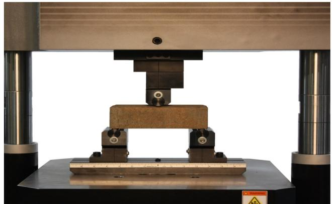
**Modulus of Rupture being tested on a refractory sample.**
