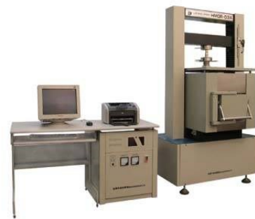
Typical Hot Modulus of Rupture Testing Apparatus
