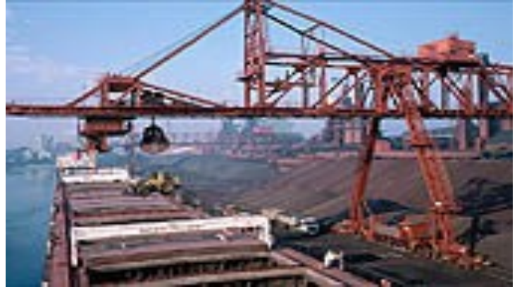
Taconite pellets refined from iron ore in Northern Minnesota are unloaded at Gary, Indiana for processing into iron and steel. U.S. Steel and other domestic companies, have their own mines and processing plants, reducing their dependence on outside sources.
