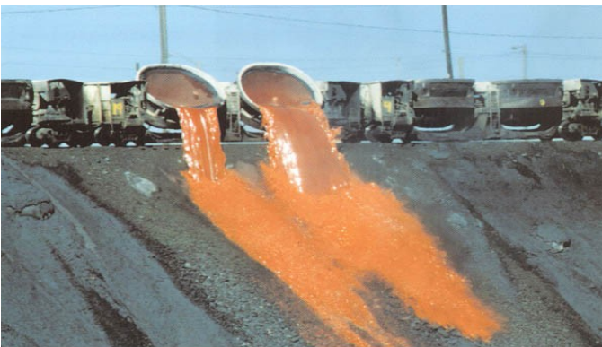
Blast furnace slag being dumped into a pit. Much of this is allowed to cool and is processed into aggregate for bedding for roads.
